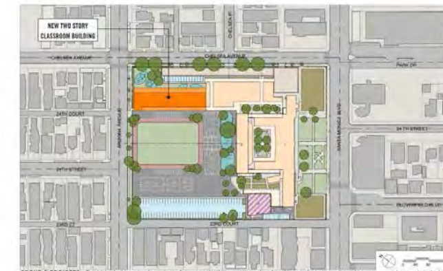
GROUP 2 PROJECTS Could include a new two story classroom building with early education and kindergarten classrooms and associated play area at the ground floor, upper elementary classrooms at the second floor.
